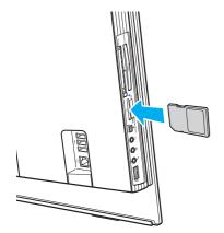
**3** Carefully slide the memory card into the slot until it clicks into place. Do not force the card into the slot.
