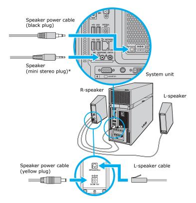
4 Insert the mini stereo plug of the cable that is attached to the right speaker, into the Headphones jack, located on the back panel of your computer.
