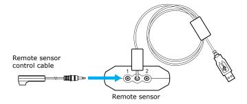
2 Place the remote sensor control above the set-top box's infrared port.
