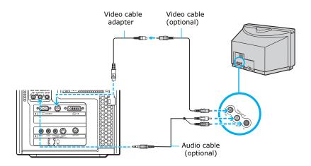
The video cable adapter is not necessary, if you use an S-video cable to connect your TV to the computer's TV out (S-video/video) jack.
