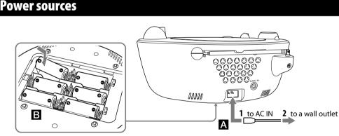
Connect the AC power cord A or insert six R14 (size C) batteries (not supplied) into the battery compartment B.
