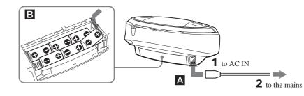
Connect the mains lead  $\blacksquare$  or insert six R20 (size D) batteries (not supplied) into the battery compartment  $\blacksquare$ .
