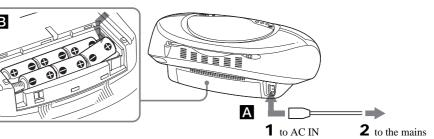
Connect the mains lead A or insert six R20 (size D) batteries (not supplied) into the battery compartment B.
