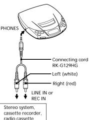
• Before you play the CD, turn down the volume of the connected equipment so as not to damage the connected speakers.
