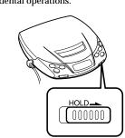
Slide HOLD in the direction of the arrow. When you press any button, "Hal d" appears in the display and you cannot operate the
