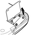
When to replace the dry batteries When the battery becomes weak, indication appears in the display. If the "L 🛛  $b\partial tt$  " appears in the display, replace all the batteries with new ones, because the batteries are used up.
