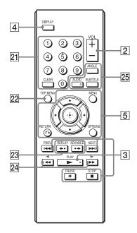
The VOL +, number 5, ▶ and AUDIO buttons have a tactile dot. Use the tactile dot as a reference when operating the player.
