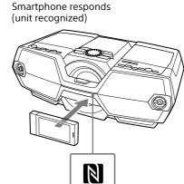
After being recognized by the unit, follow the on-screen instructions displayed on the smartphone, and complete the procedure for BLUETOOTH connection. When the BLUETOOTH connection is established, the BLUETOOTH indicator (8)
