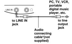
For a PC: use a cable which fills the connector of your PC.
