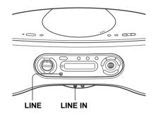
1 Connect the LINE IN jack to the line output jack of the portable digital music player or other components using an audio connecting cable (not supplied).
