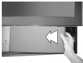
Remove the front panel without moving the set.
