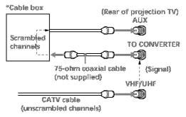
For this set up, you can switch between scrambled channels (through your cable box), and normal (CATV) channels by pressing ANT on your remote control.
