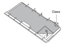
4 Attach the air filter cover to the unit.
