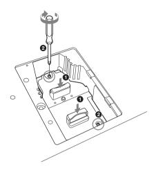
**5** Close the lamp cover and tighten the 1 screw.
