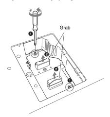
4 Insert the new lamp all the way in until it is securely in place. Tighten the 2 screws.
