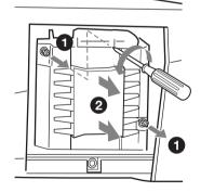
5 Insert the new lamp all the way in until it is securely in place (1). Tighten the two screws (2).
