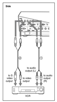
Audio connecting cable (not supplied) For stereo equipment use both the L and R jacks.
