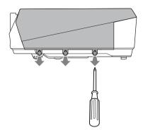
**3** Remove the lamp cover by lifting it forward with the fingers placed on the slit of the projector.
