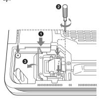
**6** Insert the new lamp all the way in until it is securely in place. Tighten the two screws. Fold down the handle.
