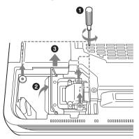
**5** While holding the handle and keeping the lamp unit horizontal, pull straight up.
