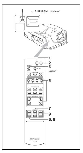
1 Set the main power switch on the left side of the projector to the upper position.
