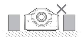
If you put something beside the ventilation holes for exhaust on the side or rear of the projector, the exhaust may be inhaled into the projector through the ventilation holes for intake, causing internal heat build-up and thereby activating the protection circuit. Be sure not to block the ventilation holes for exhaust. Leave a space of more than  $1 \text{ m} (39^{-3}/8 \text{ inches})$  around the unit.
