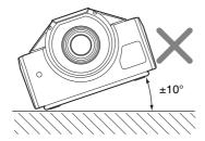
Avoid tilting the projector more than  $\pm$  10 degrees. Doing so may cause color shading or shorten the lamp life excessively.
