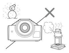
A sudden change of temperature may produce moisture condensation, causing damage to the projector. Take care with heaters or air-conditioners.
