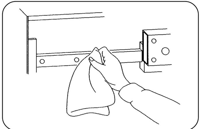
6. Apply grease to the Z unit and the ZR unit as shown in the same manner.
