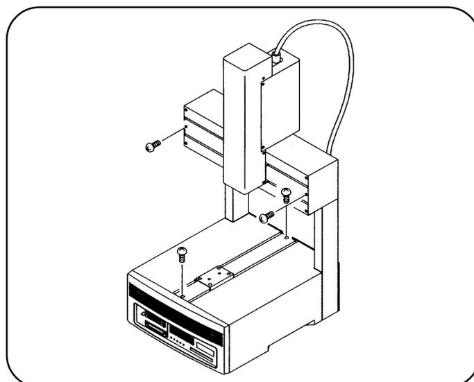
3. **Move the work table and the work unit to the ends by hand, remove the X-axis and Y-axis covers by pulling them, then remove the fallen materials such as screws.**
