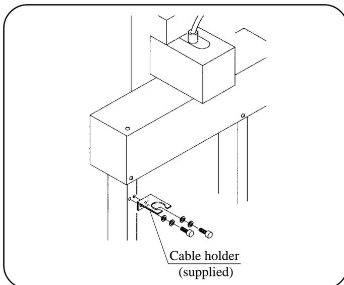
**7. Fix the cable clamp of the cable to the cable holder.**
