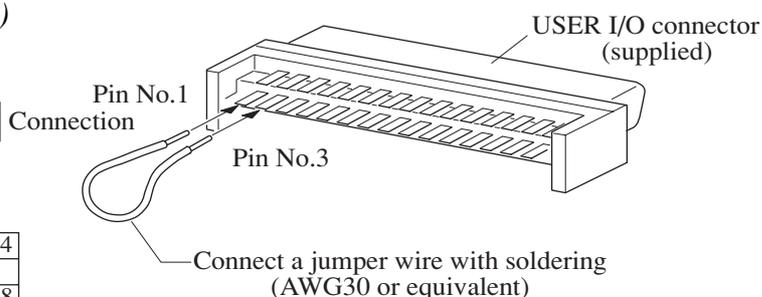
\* Connect a jumper wire to the USER I/O connector (supplied), with soldering, attach the connector supplied (accessory) to the connector.
