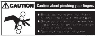
Be cautious not to pinch your hands or fingers into the units moving parts. Before you perform any maintenance and/or check, disconnect the unit from the main power supply.
