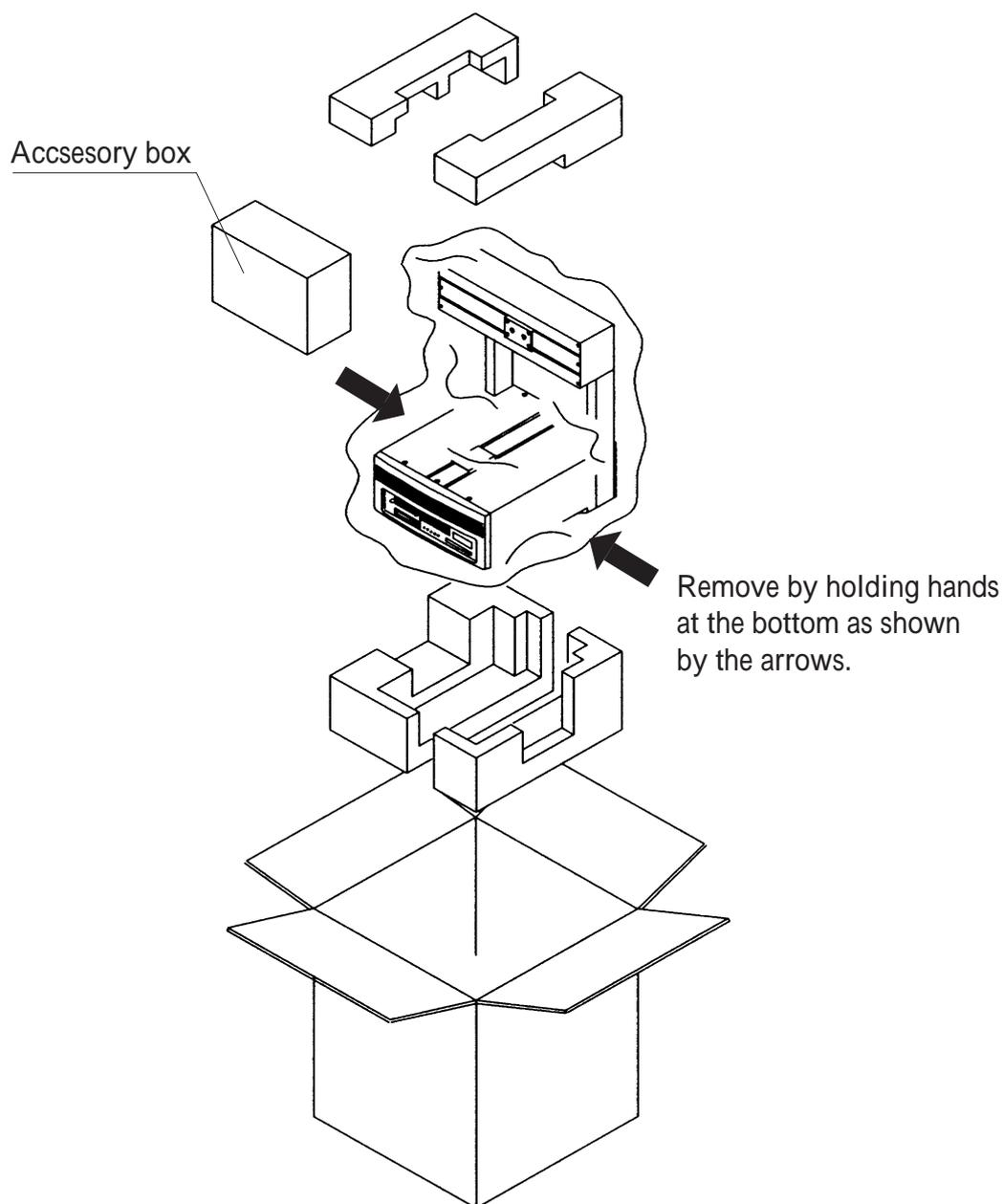
When the machine is unpacked, make sure the following items are in the package.
