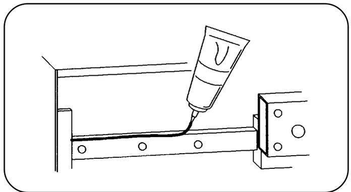
5. **Move the work table and the work unit to the left and to the right several times to spread the grease over the length of each rail.**
