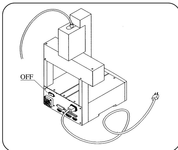
2. Remove the screws securing the X-axis and Y-axis cover, and also the front cover of Z unit and ZR unit (also Z-axis cover for the 3 axes specification).
