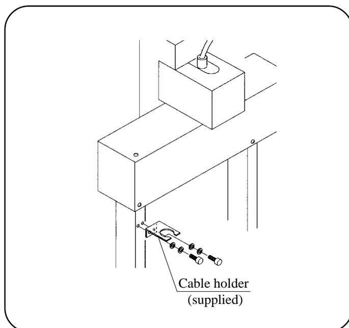
**5. Fix the clamp of the cable on the cable holder.**
