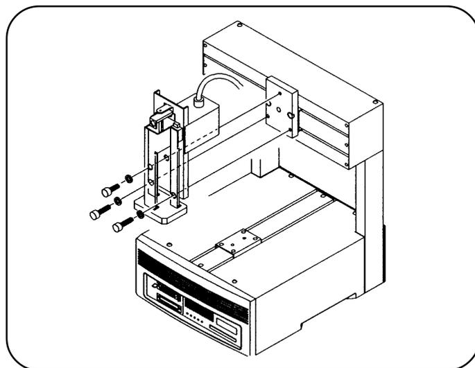
**4. Attach the removed front cover. (Four positions)**
