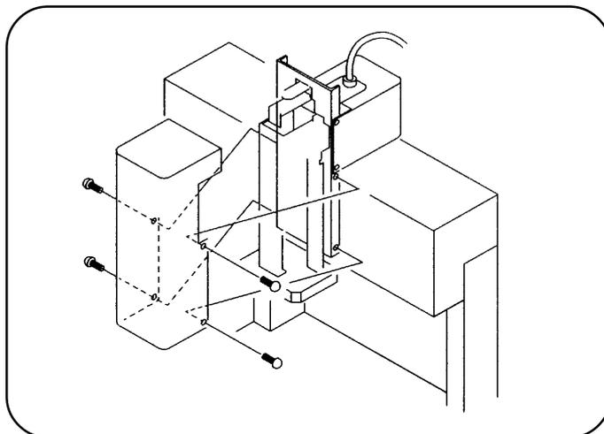
**5. Connect the connectors to the Z-/ZR-unit connectors.**
