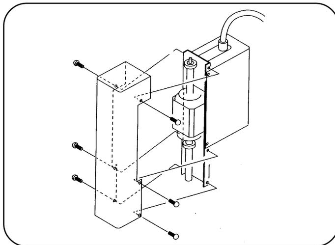
2. Fix the ZR-unit to the mounting plate. (Four positions)
