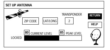
To determine the elevation and azimuth settings for the satellite antenna, select ZIP CODE or LAT/LONG.
