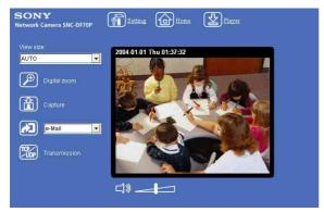
When the main viewer is correctly displayed, the IP address assignment is completed.
