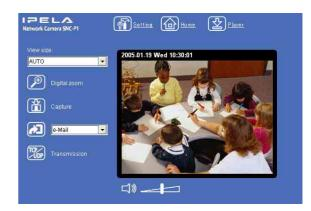
2 Select the frame rate (only when the camera Video mode is set to **JPEG**).
