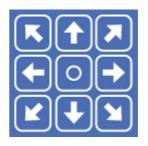
Observe the monitor image and click the arrow button indicating the direction in which you want to move the camera. The camera moves and the monitor image follows. Hold down the arrow button to move the direction of the camera continuously.
