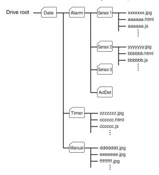
A \_\_\_\_\_ represents a folder created automatically. The Date folder has a 6-digit folder name consisting of the lower two digits of year (2 digits), month (2 digits) and date (2 digits). The Sensor 1, Sensor 2, Sensor 3 and Act Det (activity detection) folders correspond to alarm modes. The Timer folder corresponds to the periodical recording mode. And, the Manual folder corresponds to the manual mode.
