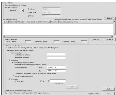
In the Camera IP Setup window, you can search for cameras on the same network by MAC address and configure their IP addresses all at once.
