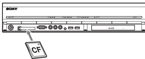
When ejecting a CompactFlash card, press the eject button on the left of the card slot.
