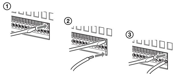
Repeat this procedure to connect all required wires.
