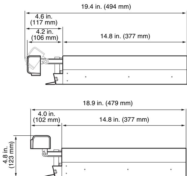
You can set up the NSR in a rack mount or on a flat surface. If you plan to set it up on a flat surface, you must attach the supplied rubber feet to the bottom of the chassis.
