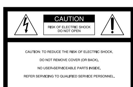
This symbol is intended to alert the user to the presence of uninsulated "dangerous voltage" within the product's enclosure that may be of sufficient magnitude to constitute a risk of electric shock to persons.
