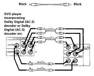
\* It is possible to use a pair of audio cords instead of two monaural audio cords to connect to the 5.1 CH INPUT CENTER and 5.1 CH INPUT WOOFER jacks.
