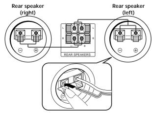
Be sure to connect matching speaker terminals (e.g., use the solid-color wire to connect + to +, and use the striped wire to connect – to -). If the connections are reversed (+ to -), the sound will lack bass.
