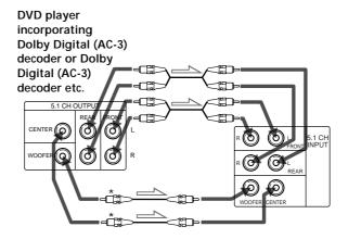
\* It is possible to use a pair of audio cords instead of two monaural audio cords to connect to the 5.1 CH INPUT CENTER and 5.1 CH INPUT WOOFER jacks. Setting the Dolby Digital (AC-3) decoder Specify the speaker type in the decoder's display as below:
