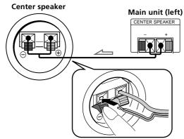
Be sure to connect matching speaker terminals (e.g., use the gray wire to connect + to +, and use the striped wire to connect – to –). If the connections are reversed (+ to –), the sound will lack bass.
