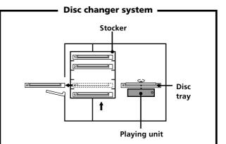
The disc changer consists of a playing unit, trays which hold the discs, and a stocker which transports the discs on their trays to the disc slot and the playing unit.
