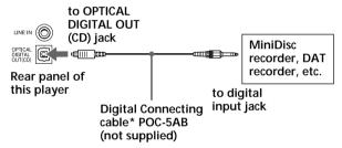
Select a connecting cable depending on the type of the digital input jack of the recorder to be connected. For details, refer to the instruction manual of the component to be connected. The OPTICAL DIGITAL OUT (CD) jack of this player is square-shaped jack.
