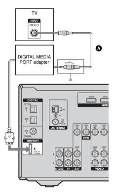
\* The type of connector varies depending on the DIGITAL MEDIA PORT adapter. For details, refer to the operating instructions supplied with the DIGITAL MEDIA PORT adapter.
