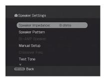
Press ♣/♦ repeatedly to select "4 ohms" or "8 ohms" depending on the speakers you are using, then press ⊕.
