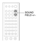
Press SOUND FIELD +/- on the remote repeatedly until "C.ST.EX A (or B, C)" appears on the front panel display.
