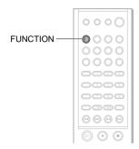
Press FUNCTION repeatedly until VIDEO 1 or VIDEO 2 that you connected the unit to appears in the front panel display.
