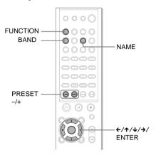
Press FUNCTION repeatedly until FM or AM appears in the front panel display.
