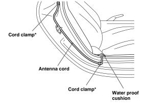
• Clean the mounting surface before installing the cord clamp. · Leave the installed cord clamp for 24 hours before installing the cord. Otherwise, the cord clamp may come off because of weak attachment.
