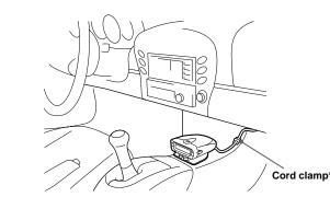
• Clean the mounting surface before installing the cord clamp. • Leave the installed cord clamp for 24 hours before installing the cord. Otherwise, the cord clamp may come off because of weak attachment.
