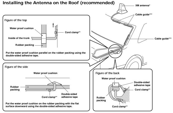
\* Be sure to install the antenna firmly on a flat surface. Do not install on the corner of the roof.
