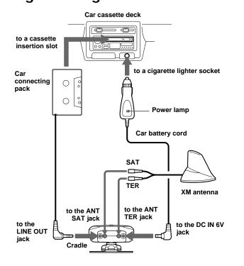
When the electric power is supplied to the car battery cord, the power lamp lights up.
