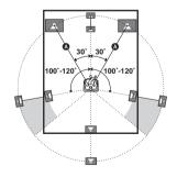
When placing two surround back speakers (The angle **3** should be the same)
