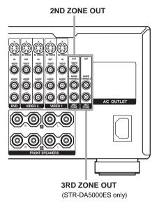
You can select analog audio/video signals for output to the 2nd zone or audio signals for the 3rd zone (STR-DA5000ES only). For details on the connection, see page 53.
