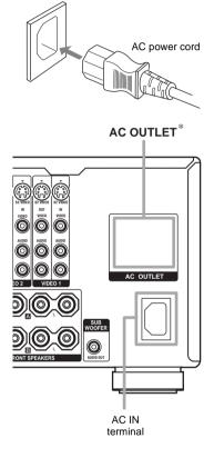
\* The configuration, shape, and number of AC outlets vary according to the area code.
