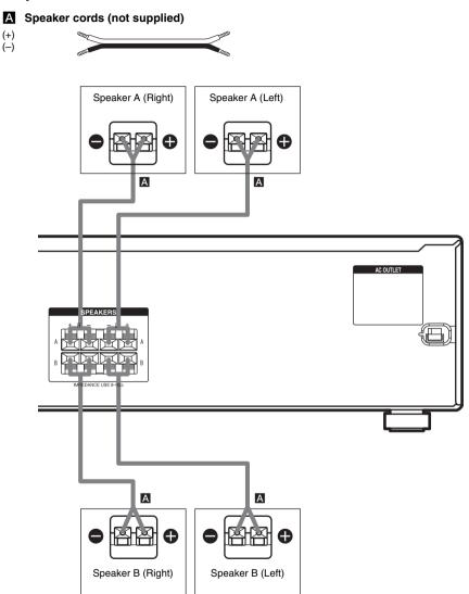
\* If you have an additional speaker system, connect them to the SPEAKERS B terminals. You can select the speakers you want to use with the SPEAKER A and SPEAKER B buttons. For details, see "Selecting the speaker system" (page 17).
