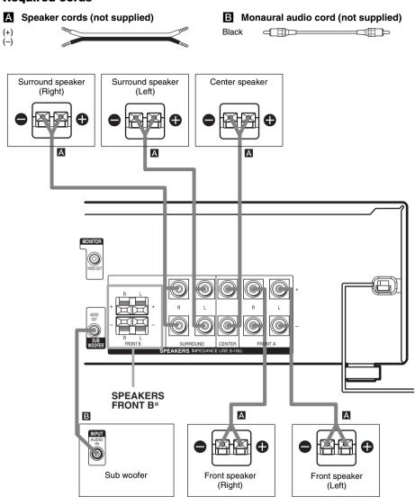
\* If you have an additional front speaker system, connect them to the SPEAKERS FRONT B terminals. You can select the front speakers you want to use with the SPEAKERS (OFF/A/B/A+B) button. For details, see "Selecting the speaker system" (page 36).
