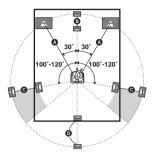
When placing two surround back speakers (The angle 🕒 should be the same)
