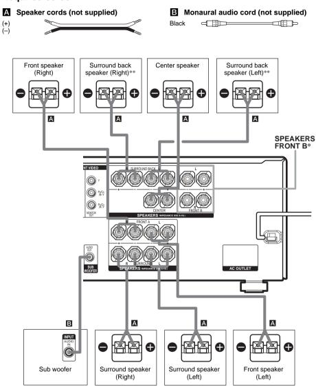
\* If you have an additional front speaker system, connect them to the SPEAKERS FRONT B terminals. You can select the front speakers you want to use with the SPEAKERS (OFF/A/B/A+B) button. For details, see "Selecting the speaker system" (page 43).
