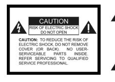
The lightning flash with arrowhead symbol is intended to alert the user to the presence of uninsulated "dangerous voltage" within the product's enclosure that may be of sufficient magnitude to constitute a risk to persons.
