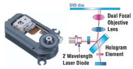
**Precision Drive™ 2 System** Past generations of Precision Drive technology were only able to compensate for warped discs by moving the entire optical block, which took more time and limited the amount of correction possible.
