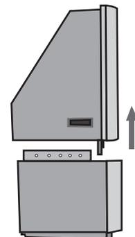
**IMPORTANT:** Avoid contacting the CRT assembly when separating or reattaching the top and bottom portions of the cabinet.
