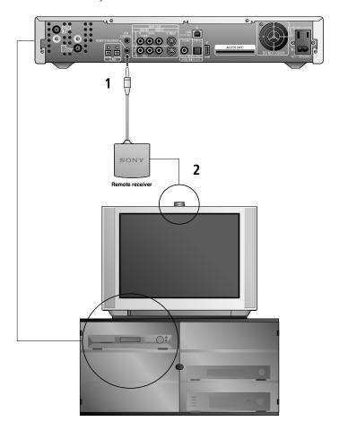
**2** Place the Remote Receiver on top of the TV, with the IR window facing out as shown.
