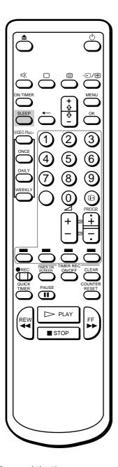
You can automatically switches the video TV into standby mode after a selected time period.
