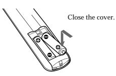
Check the polarities and position two R6 batteries correctly.
