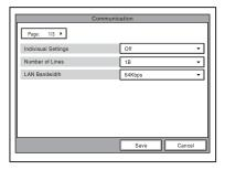
Select the LAN bandwidth to be used for multipoint videoconferencing in "LAN Bandwidth" on page 1 of the Communication Setup menu.
