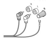
**2** On the mixer, connect the red plugs and white plugs on the other end of each audio cord to the PHONO R and PHONO L INPUT jacks, respectively, for CH-1 and CH-2, as shown below.
