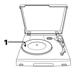
Place the rubber mat on the platter. To make sure it operates properly, rotate the platter clockwise once or twice with your hand.
