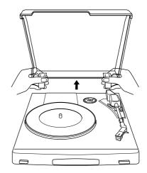
**2** Remove the lid, and set the voltage selector to the local power line voltage using a screwdriver.
