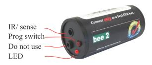
The IR/ sense socket is output for the IR-emitter that sends IR to the device to be operated. In some cases this socket is also used for sensing purposes. Often the BeeLINK2 controller needs to know if the device is powered up or not. In some cases this socket is used for other serial communication like RS-232.
