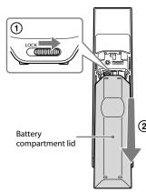
2 Insert the four supplied LR6 (size AA) batteries.
