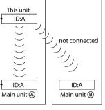
1 Place the S-AIR main unit to be paired near this unit. Pair the main unit with the remote
