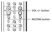
Press the VOL +/- buttons to control the volume, and the MUTING button for silence. When you select a visual component, the TV's volume will be controlled; when you select an audio component, the amplifier's volume will be controlled.
