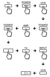
You can program up to 16 consecutive steps on each of the SYSTEM CONTROL buttons (1 – 4), including the initial step of pressing switch to a Component Select button.
