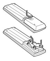
Insert the batteries negative-andfirst through the guide clamp within each compartment as shown above.
