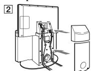
Depending on the connected equipment cords, the back covers may not attach properly. In this case, try other cords, or use the system without the back covers
